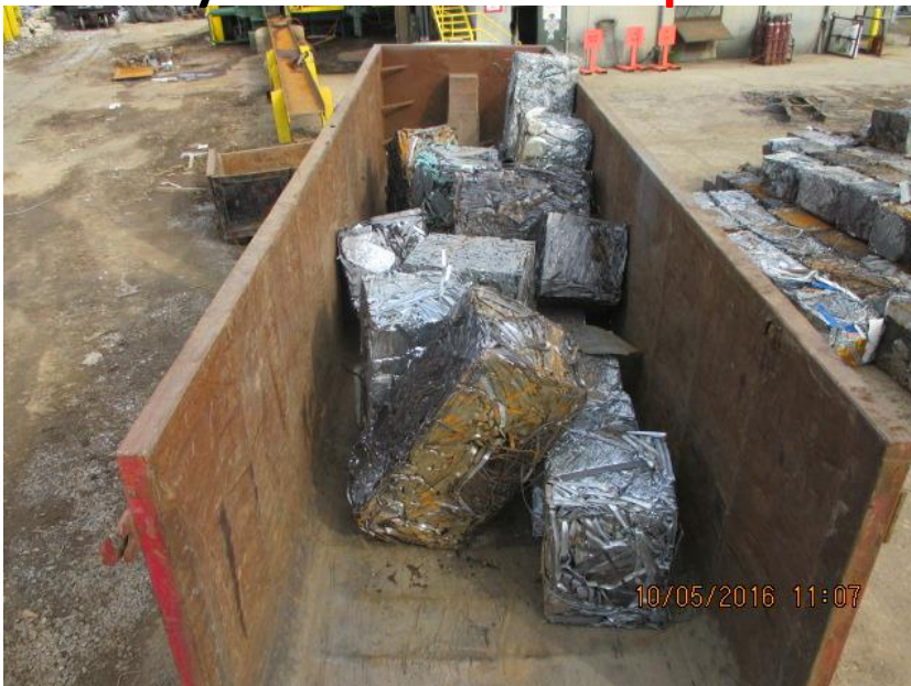
Unevenly loaded trailer – Tip over Risk
